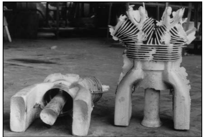
Above: Raw Aluminum Heads, Cast by Menasco (San Diego Aerospace Museum)
