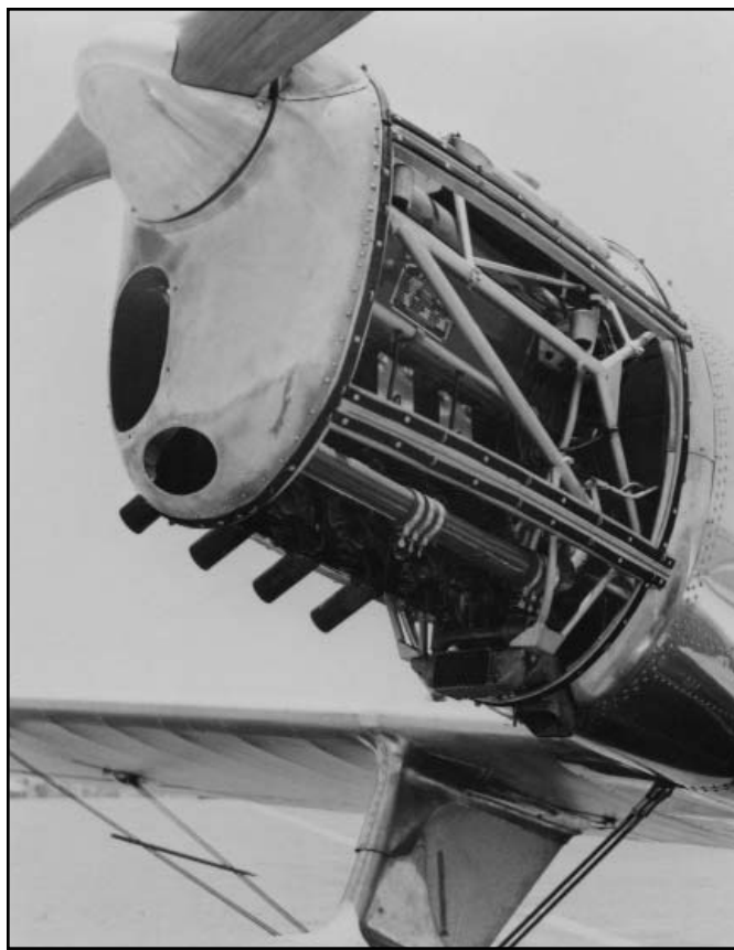
150 hp Menasco C4S in Ryan ST-A Special (Teledyne Ryan Aeronautical via Ev Cassagneres)
