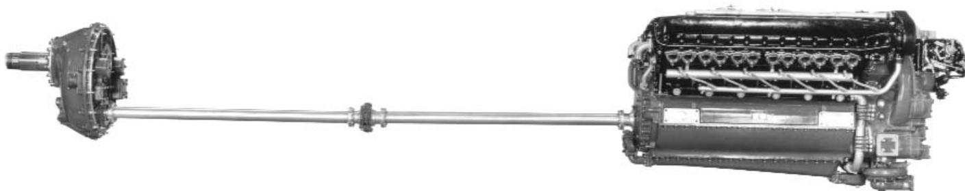
Fig 10. Allison V-1710-E as used in the Bell XP-39
