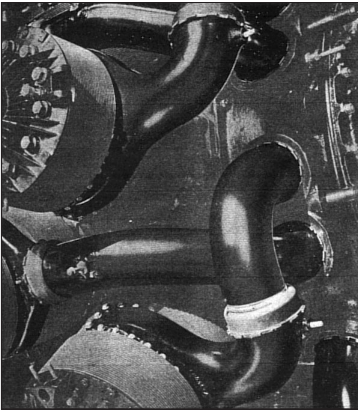
Fig. 5. Much Improved Centaurus Induction Pipes
