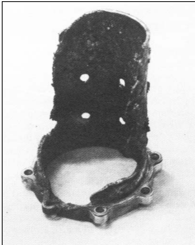
Figure 21. MOV Inlet Sleeve After Test 9001-225. (photo No. 307-971)
