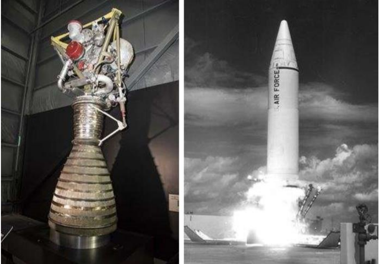
Rocketdyne LR79 (S-3D) engine on display at NMUSAF, and ignites during a Jupiter test launch at Cape Canaveral, Florida, in 1960
