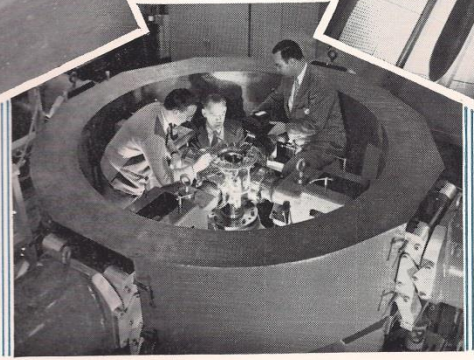
No. 1—This is one of the highly specialized tools and facilities which expedite the manufacture of Curtiss Monocoque Hollow Steel blades. The red-hot blade is placed in the blade "blow-up die". Nitrogen under high pressure inflates the hollow shell to fit the form of the die, thus imparting the correct airfoil section and pitch distribution.
