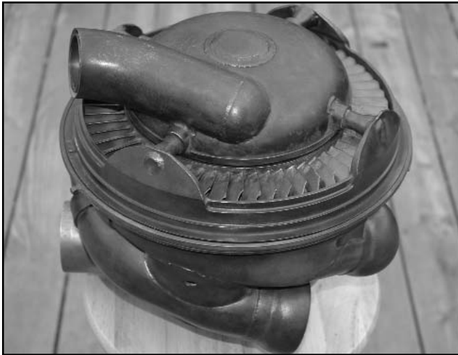
Fig. 7. PRT with Cooling Cap Installed
