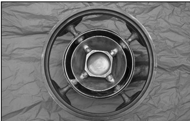
Fig. 9. Underside of Cooling Cap
