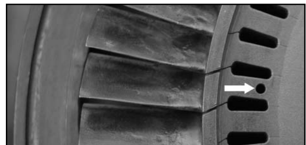
Fig. 5. Turbine. Arrow indicates bucket triggering hole.
