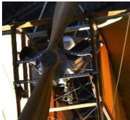
Anzani 3-cylinder "fan engine" in Bleriot monoplane (Robeson photo)
