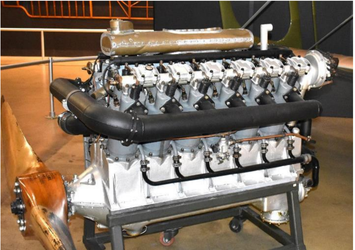
Packard Liberty 12A with turbosupercharger, at port wing of LUSAC. (Robeson photo)
