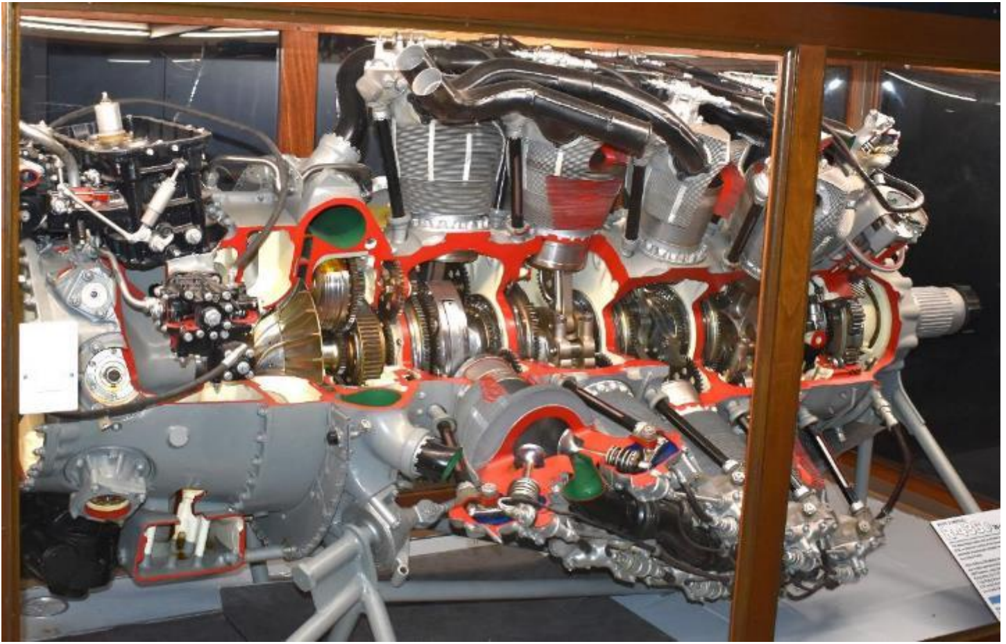
PW R-4360 Wasp Major (motion activated, starboard side of C-124) (Robeson photo)
