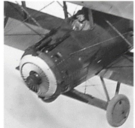
Salmson Z-9 installed in Salmson 2 WWI aircraft. Note louvered radiator in front of exhaust manifold. (Wikipedia photo)
