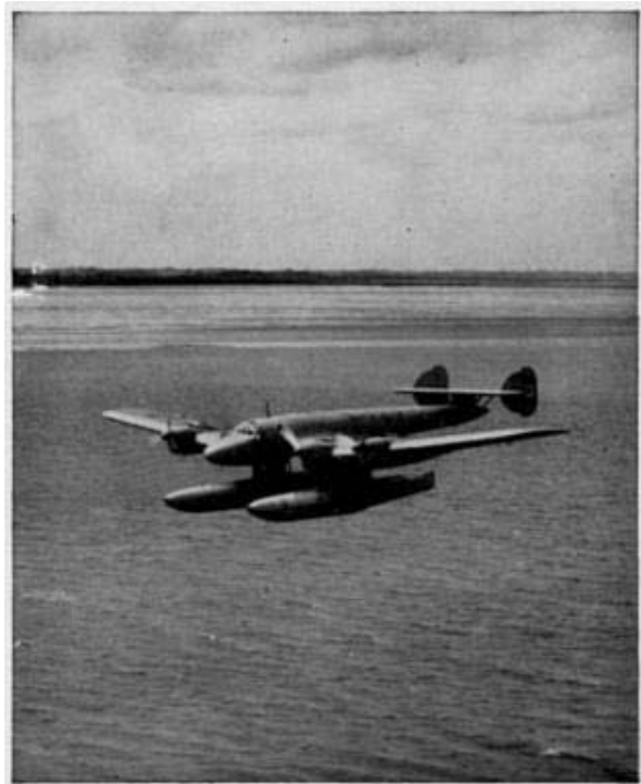
Fig. 57.—Blohm & Voss Ha 139 Diesel-engined transatlantic mailplane.
