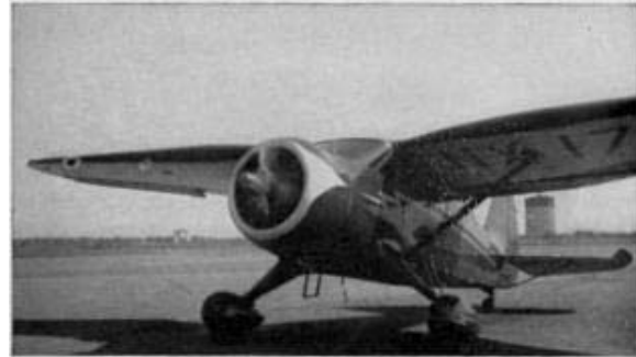
Fig. 62. —Privately-owned Stinson Reliant powered with Guiberson A-1020 Diesel.
