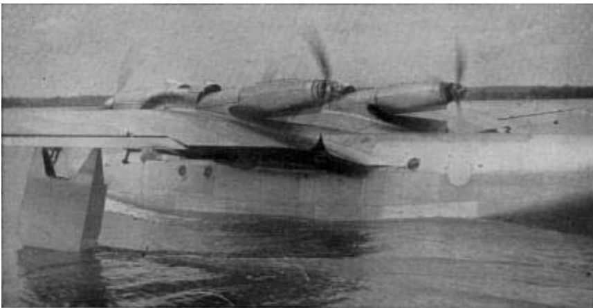
Fig. 52.—Dornier Do 26 flying boat with rear engines raised for take-off.
