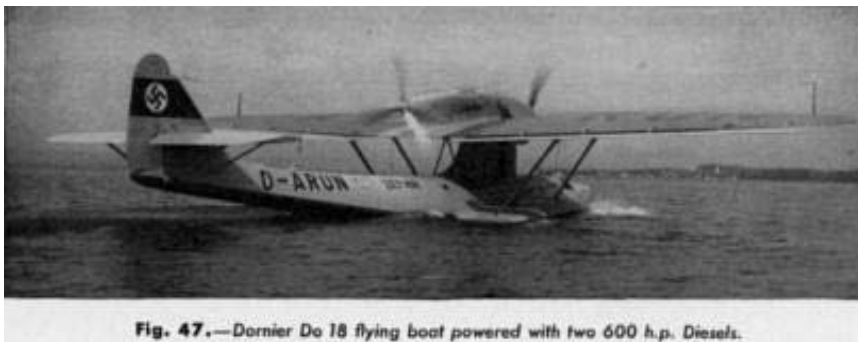
Fig. 47.—Dornier Do 18 flying boat powered with two 600 h.p. Diesels.
