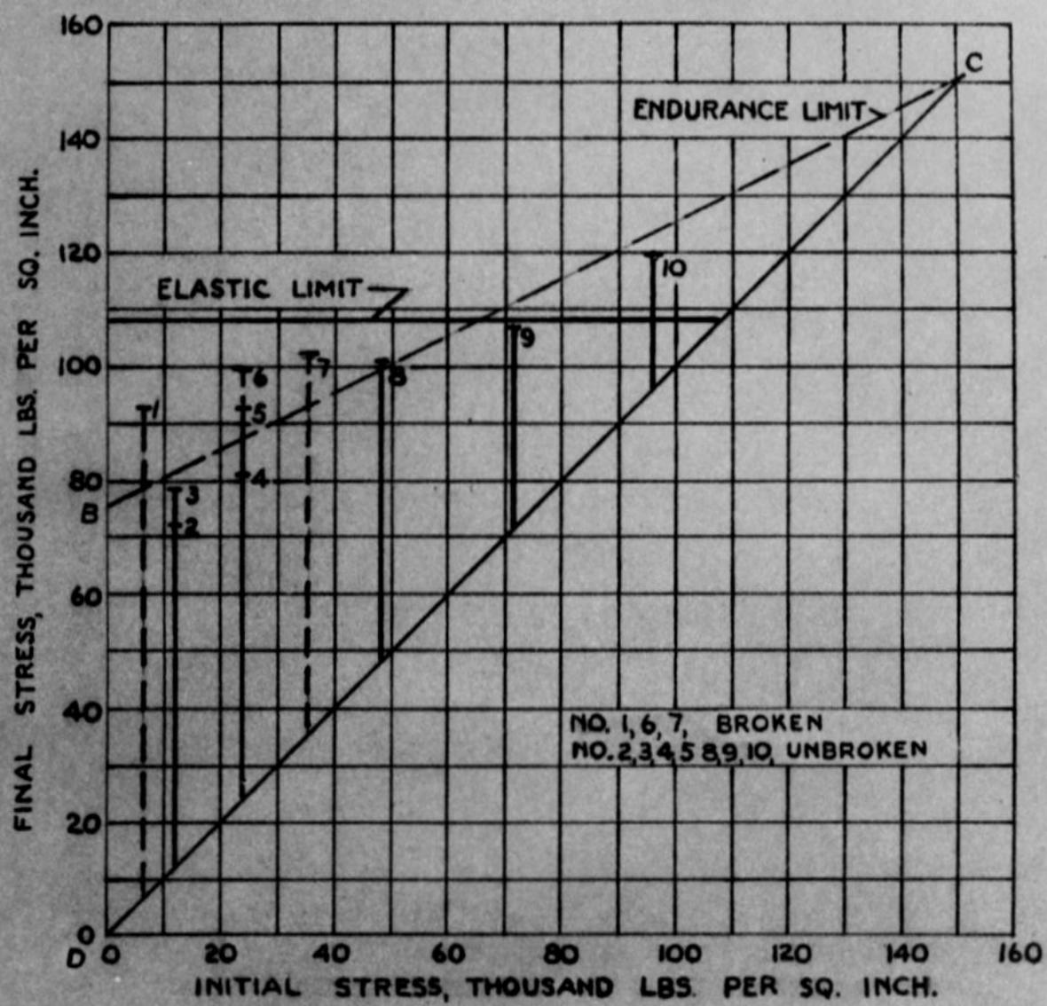
**FIG. - FATIGUE LIMIT DIAGRAM FOR
