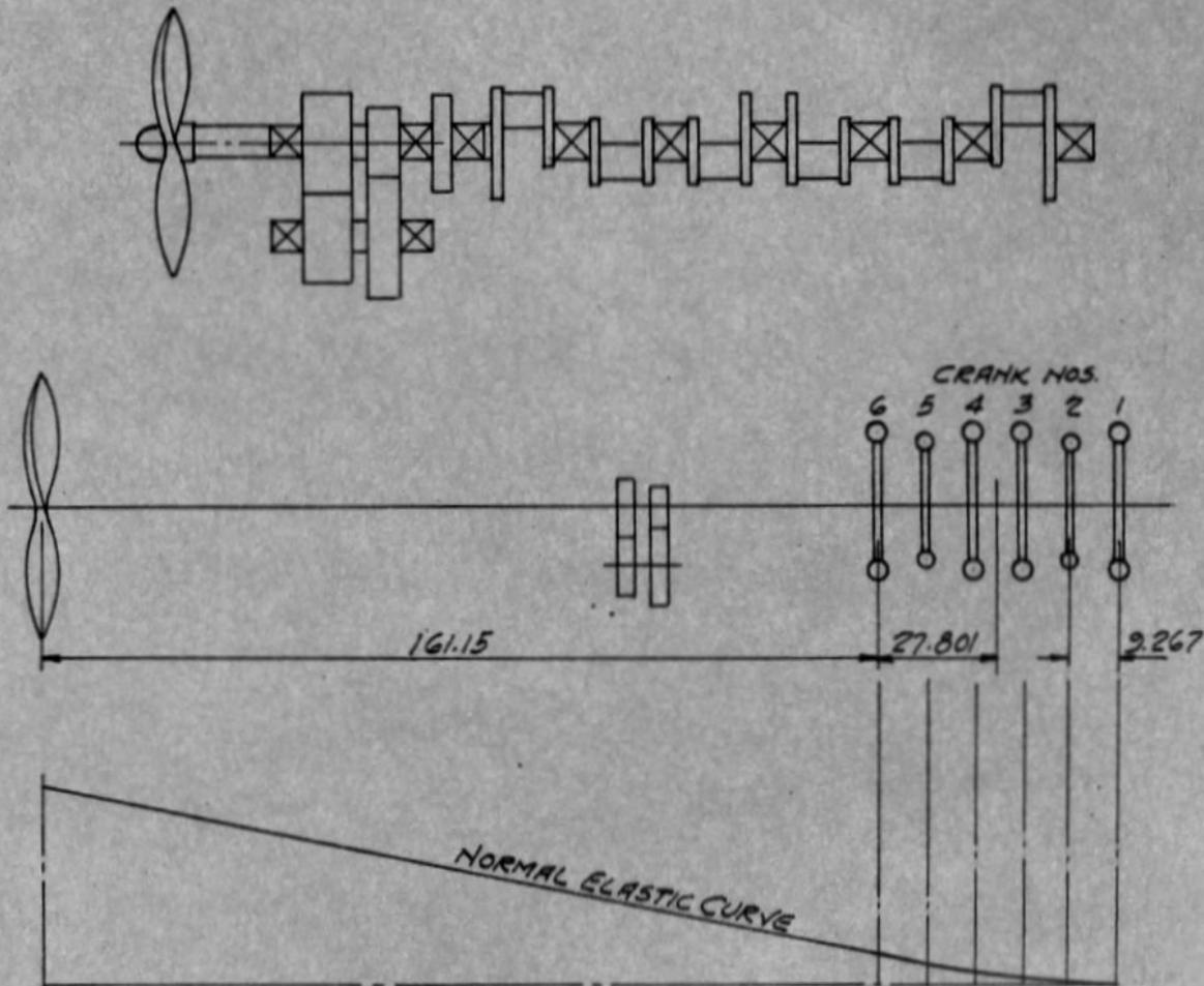
The static deflection curve for a 12-cylinder, 7 bearing crankshaft system, such as the Continental O-1430-1, may be calculated by assuming the respective masses as concentrated on each crank and calculating the necessary force to accelerate them.
