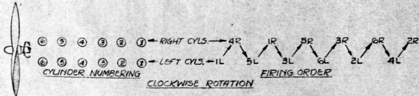
CRANK ARRANGEMENT, CYLINDER NUMBERING AND FIRING ORDER - CONTINENTAL O-1430-1 ENGINE
