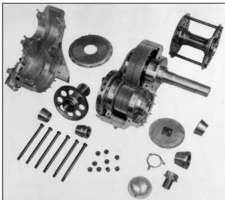
W-1A stand-alone reduction gear designed and built by the Allison Engineering Co. of Indianapolis under a contract initiated in early 1921. The gear passed acceptance in about June of 1923. It is not known to have ever been installed on an engine that flew.
