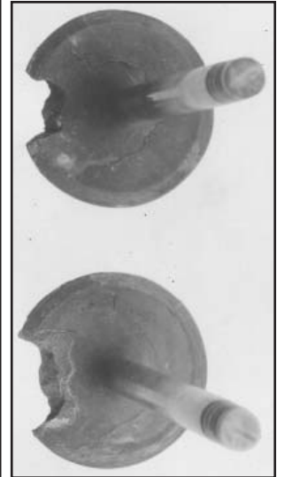
Burned Exhaust Valves from AS 95057
