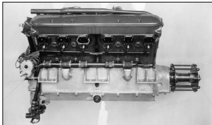
Wright T-3, the last of the Wright "T" series. The T-2 and T-3 engines were used primarily by the Navy for Martin torpedo bombers, powering a total of about 65 of these types.
