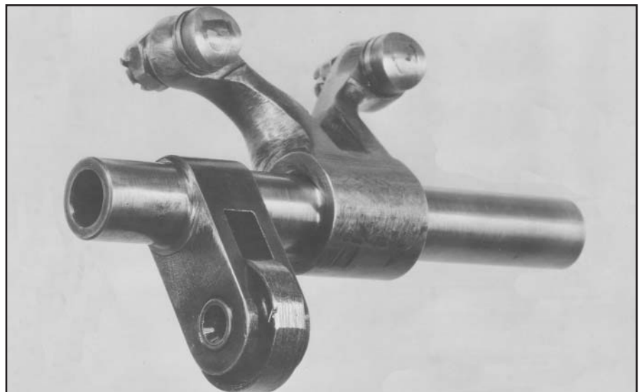
Cylinder 4R Exhaust Rocker Arm from AS 94626. The roller is burned and scored.
