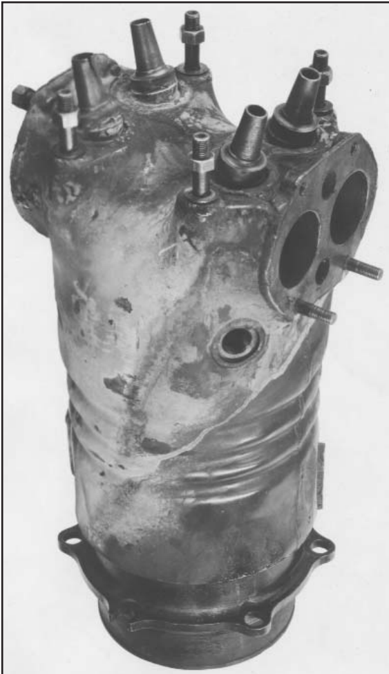
AS 95057 Cylinder after 50 Hour Endurance Test. Water leakage has deposited lime over the water jacket.
