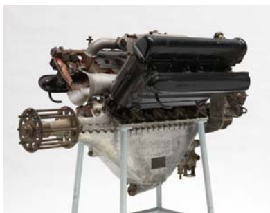
Figure 1 - H-S V-8 in Museum Victoria. Note Unusual Exhaust Pipe Manifold.
