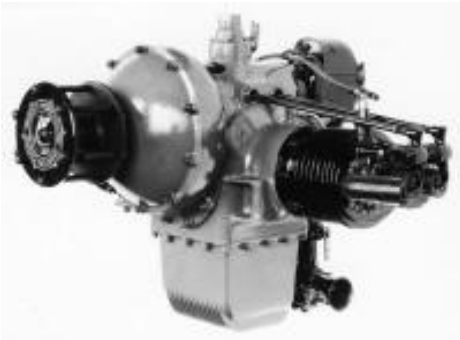
Closed-end cast iron cylinders and exposed overhead valves on the mid-1920s Wright-Morehouse opposed twin. Note the gear reduction and the deep oil sump.
