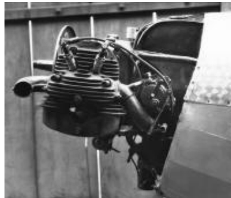
The Bristol Cherub from England is an example of an early 1930s era L-head opposed twin. The spark plugs have mica insulators and can be taken apart for servicing.
