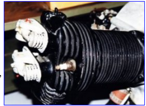
The cast aluminum head on this late 1930s Kinner engine was attached to the steel barrel by a ring of studs and nuts. The valve mechanism was enclosed (rocker covers have been removed).
